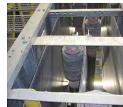
Deflection Element Umlenkstation
